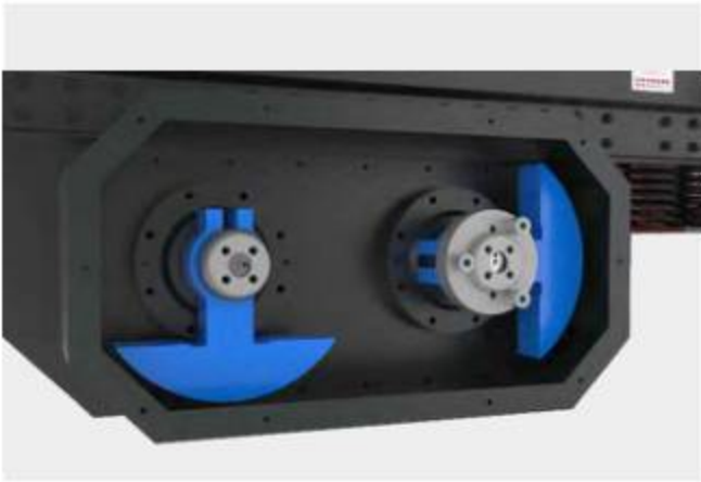
方便的振幅调节 Convenient amplitude adjustment
